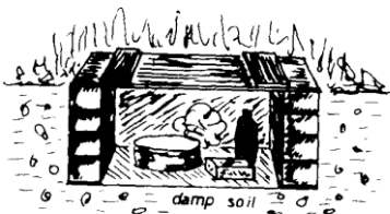
UNDERGROUND COOLING CELLAR
