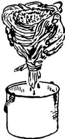
GRASS FUNNEL FOR FILTERING MUDDY WATER
